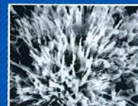
Xypex Crystallization (Mature)
